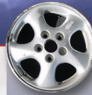
Damaged wheel with severe curb rash and gouges
